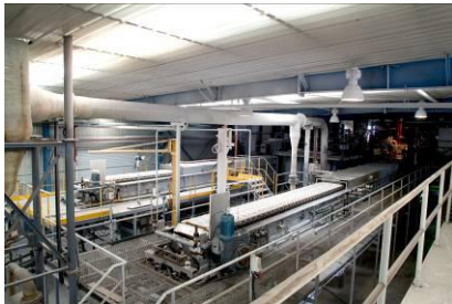
NQMg automated alloying process and casting line.
