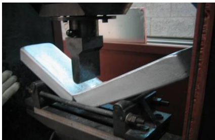
Ingot breaking for Cleanliness test (AZ91D / 8KG)
