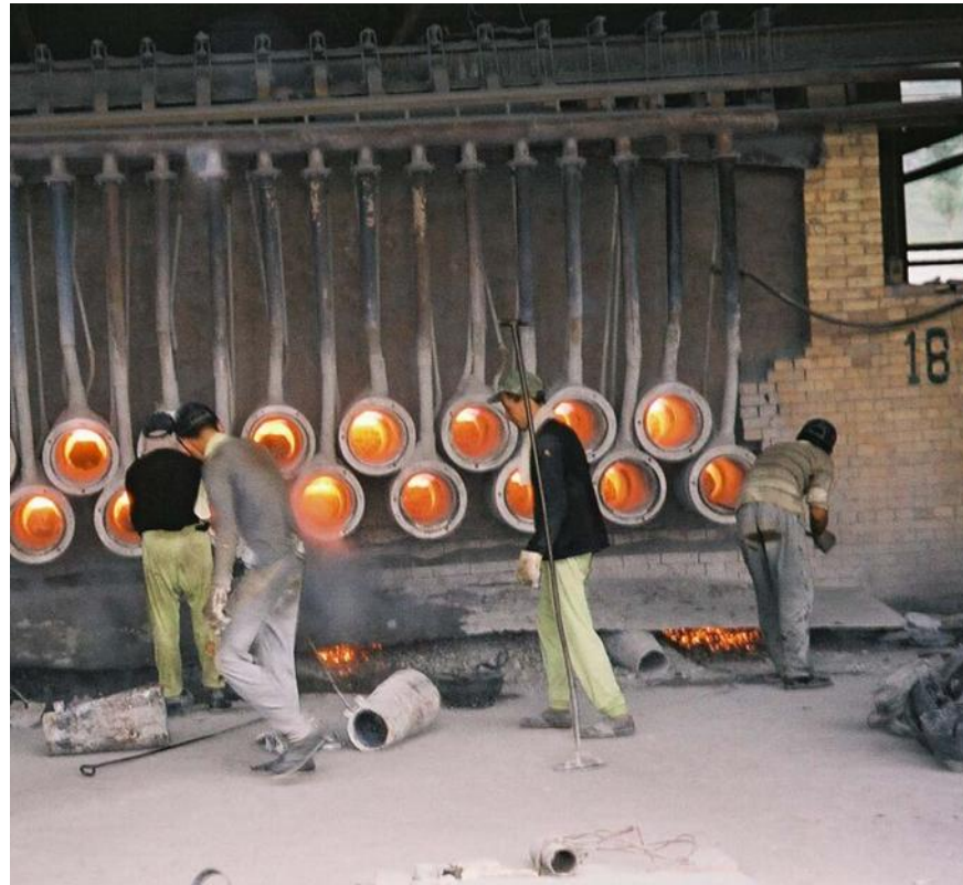
Primary magnesium plant in China (Pidgeon process) showing horizontal vacuum retorts. Produces magnesium “crowns” for further refining.
